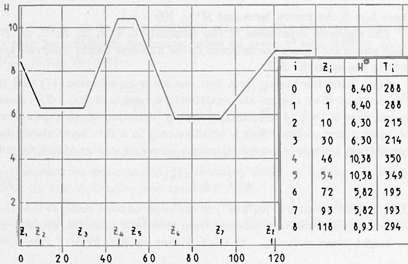
Fig. 1. - Height variation of the scale height H . The quantities H and z are in km; the temperatures T_i are in °K.
